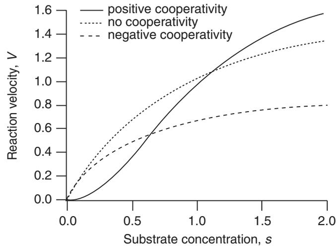
**Figure 1.3** Reaction velocity plotted against substrate concentration, for three different cases. Positive cooperativity,  $K_1 = 1000$ ,  $K_2 = 0.001$ ; independent binding sites,  $K_1 = 0.5$ ,  $K_2 = 2$ ; and negative cooperativity,  $K_1 = 0.5$ ,  $K_2 = 100$ . The other parameters are  $e_0 = 1$ ,  $k_2 = 1$ ,  $k_4 = 2$ . Concentration and time units are arbitrary.
