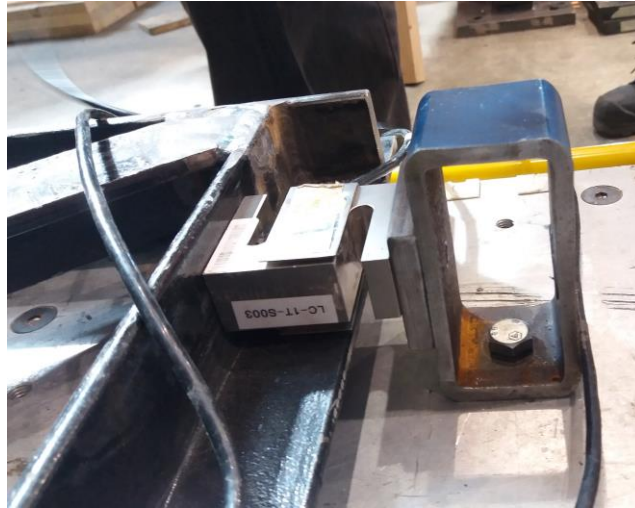
Figure 2. Set-up of the load cells.
