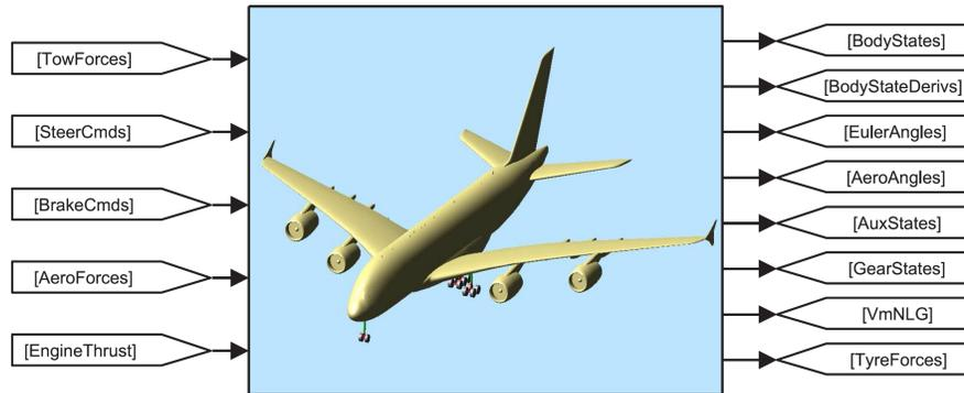
**Fig. 1** Top-level SimMechanics model of an A380. ©2012 by Airbus. Reproduced from [2].
