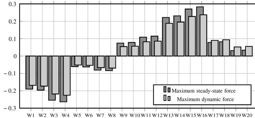
**Fig. 3** Maximum steady-state and dynamic tyre lateral load factors on main gear tyres W1–W20 for the A380 when a radius of 51 m and a velocity of 4 m/s is maintained at the nose gear. ©2012 by Airbus. Reproduced from [2].
