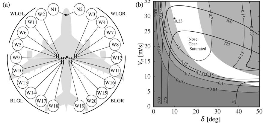
**Fig. 2** (a) Wheel numbering definition for the A380; (b) contour lines in the  $(\delta, V_n)$ -plane of the lateral aircraft load factor at the CG for the A380 at maximum ramp weight with aft CG position. ©2012 by Airbus. Reproduced from [2].
