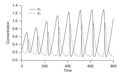
**Figure 1.8** Evolution of  $\sigma_1$  and  $\sigma_2$  for the Sel'kov glycolysis model toward a periodic solution. Parameters are the same as in Fig. 1.7.
